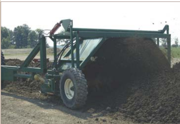
Mid-size to large composting facilities are suited for further processing of dewatered biosolids.
