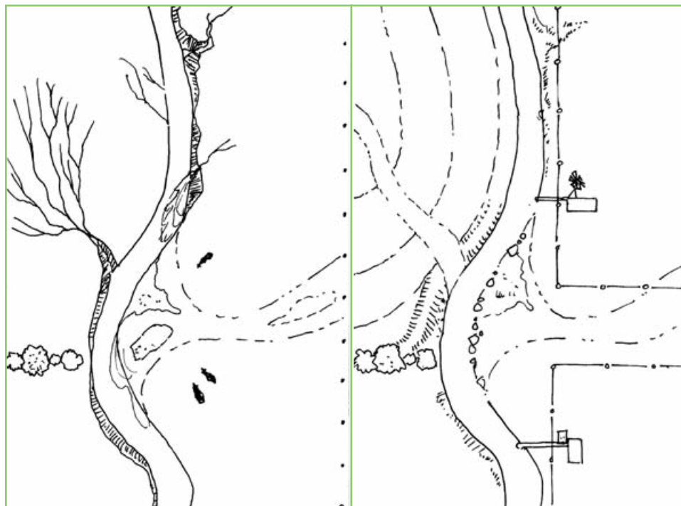
This is the “before” situation. You can see cropland erosion from the sloping field on the left of the stream. Bank degradation from intensive livestock access is also evident on the right side of the stream.
