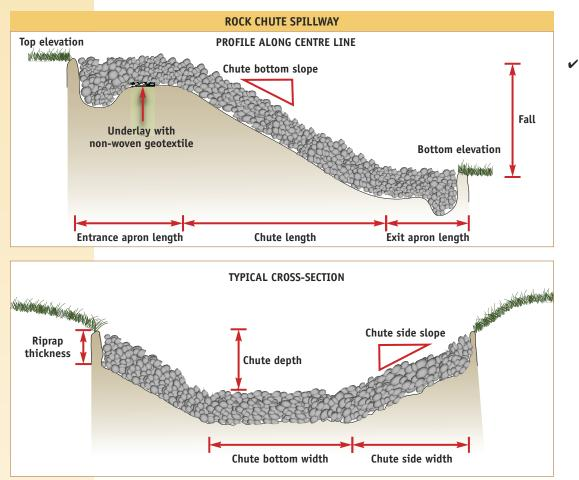
✓ <u>A rock chute</u> <u>spillway</u> is a constructed chute using angular stone (riprap) and underlaid with filter cloth. Rock chutes are often placed in riparian areas to convey concentrated surface flows safely to watercourses. As with all erosion control structures, rock chute spillways are most effective when managed as part of a soil conservation system.
