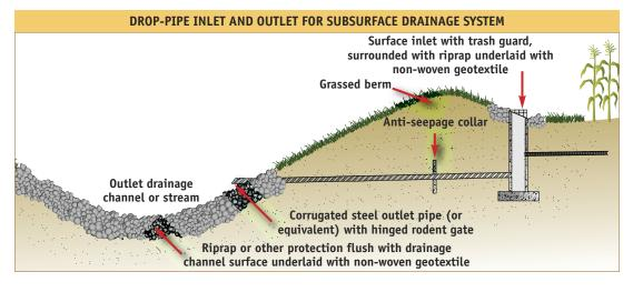
✓ A <u>large-diameter pipe (drop pipe)</u> is installed to convey water down steep slopes or high drops to prevent ponded water or concentrated flow from forming large rills or gullies.
