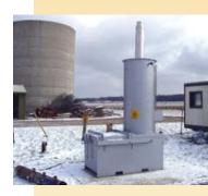
An incineration unit must have the capacity for secondary combustion to be effective and safe.
