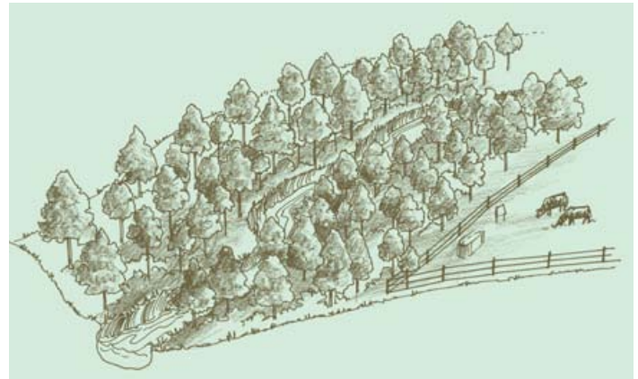
Multiple-row design: Several rows of trees and shrubs are more suitable for sites with wide valleys and steep ravine slopes.
