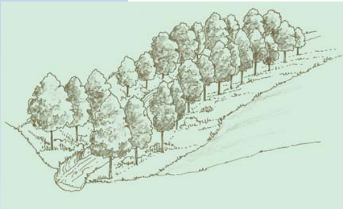
Single-row design: A combination of grass and fast-growing trees can provide considerable protection for waterways without taking up much valuable cropland.
