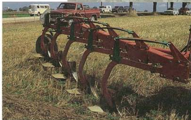
Modifying the moldboard plow will increase surface residue.
