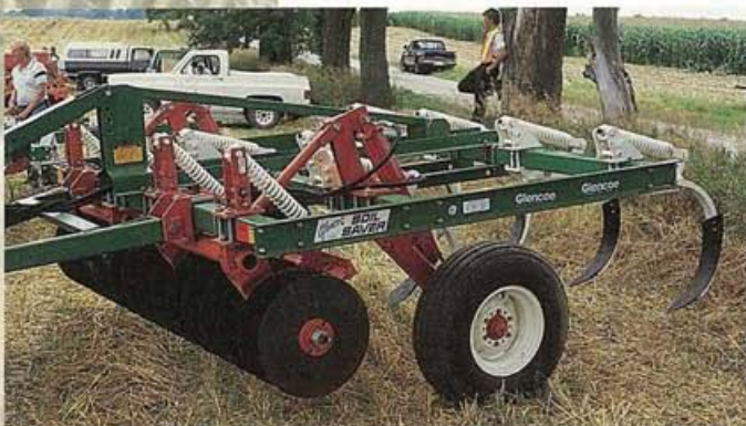
This coulters-chisel plow has a gang of coulters ahead of the chisel teeth.
