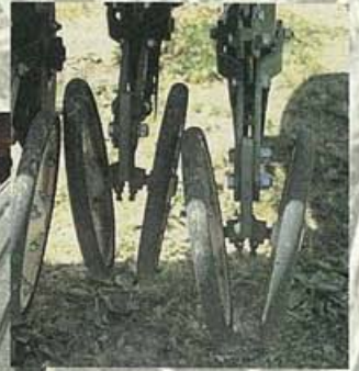
The most popular type of press wheels are the wide rubber tire style (left) and the V-style (right). Choice will depend on your soil and planting conditions.
