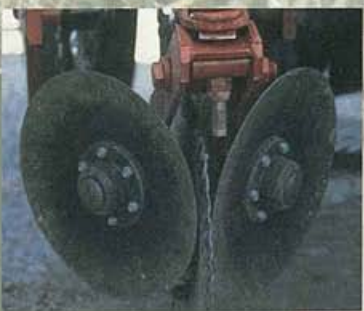
Notched trash whippers handle high residue situations easily and move the residue off the row area.
