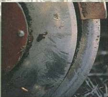
The offset double disc opener is the preferred opener for planters in high residue situations.
