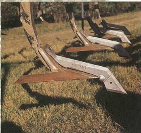
A deep banding tip on the sweep may help the chisel plow penetrate compacted, poorly structured soil.
