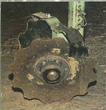
The offset double disc opener is the preferred opener for planters in high residue situations.
