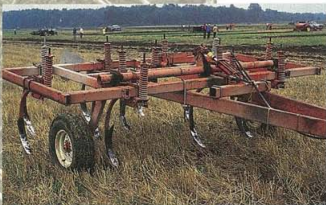
There are several types of chisel plows. This is referred to as a chisel plow with no disc/coulters on the front.
