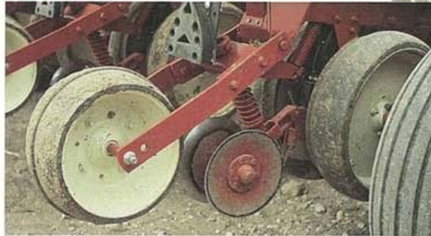
The most popular type of press wheels are the wide rubber tire style (left) and the V-style (right). Choice will depend on your soil and planting conditions.
