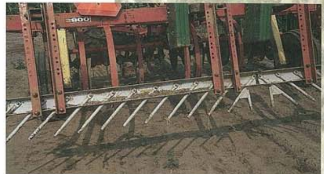
A buster bar can be added to the back of a chisel plow to help level the ridges.
