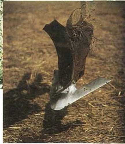
Combination twisted shovel/sweep tooth.
