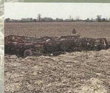
Secondary tillage should be kept to a minimum. Consider using a once over implement such as pictured to eliminate trips over the field.
