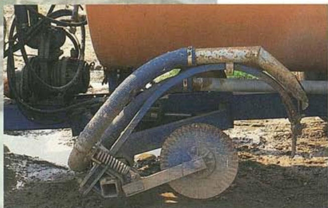
Coulters are mounted in front of injectors to cut residue.
