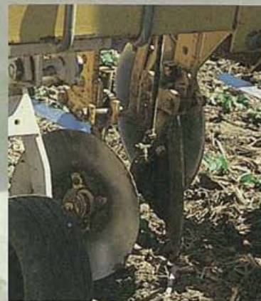
Banding nozzles on a cultivator for spot spraying in the row.
