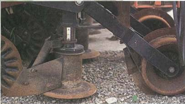
Ridge cleaners attached to the front of a conventional planter.
