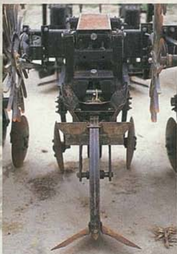
Sweeps and disc hillers on a ridge cultivator.
