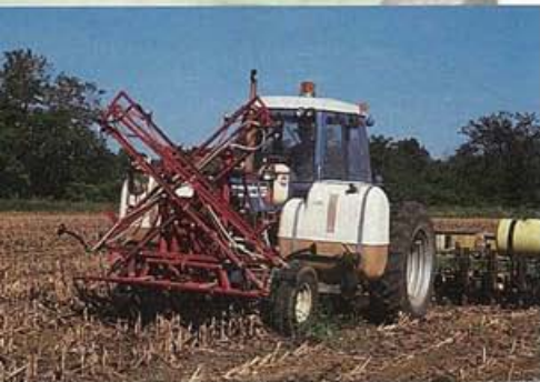
The spray boom mounted on the front of the tractor for spot spraying.
