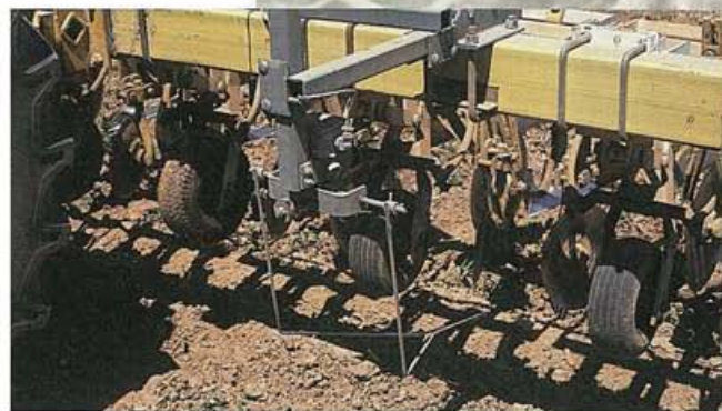
The sensing wands of a guidance system on a cultivator.
