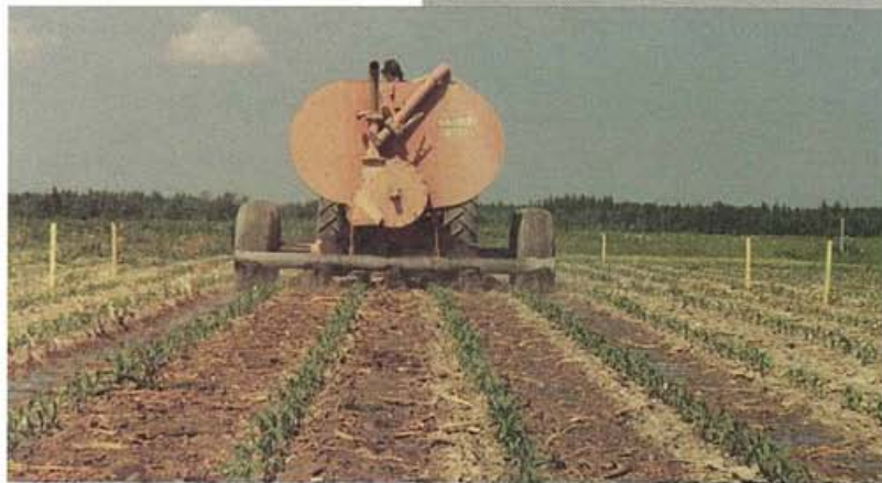
A tanker surface applies liquid manure between corn rows before inter-row cultivation.
