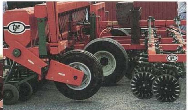
Drill with coulters caddy set-up for no-till.
