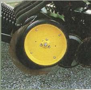
Depth gauge wheels keep the seed from being planted too deep in variable soils.
