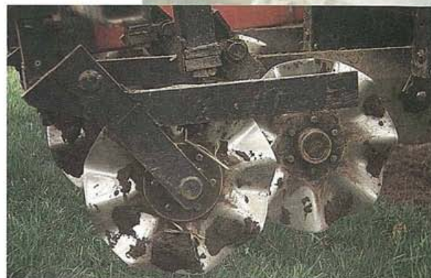
Coulters are staggered to improve residue flow.
