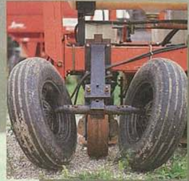
Proper alignment makes it easier to stay on the ridge.
