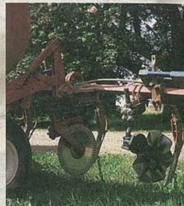
A couple of different coulters mounted on an anhydrous ammonia applicator. The chain welded on the knife helps to close the slot.
