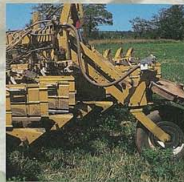
Banding nozzles on a cultivator for spot spraying in the row.
