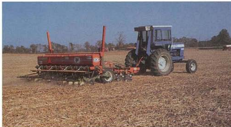
No-till drill with harrow added to improve seed coverage.
