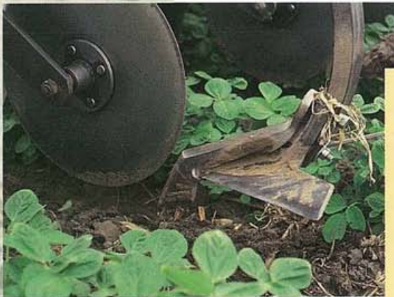
A deep banding tip on the sweep improves penetration.
