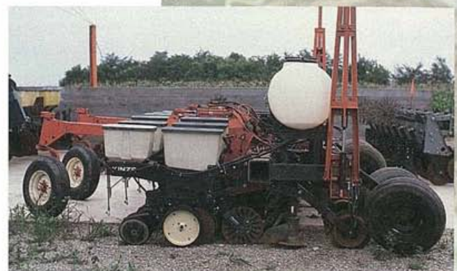
The ridge till planter used on the case study farm.
