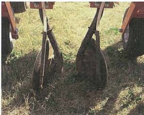
Tubes welded onto the disc furrowers of a ridge till cultivator for liquid nitrogen application.
