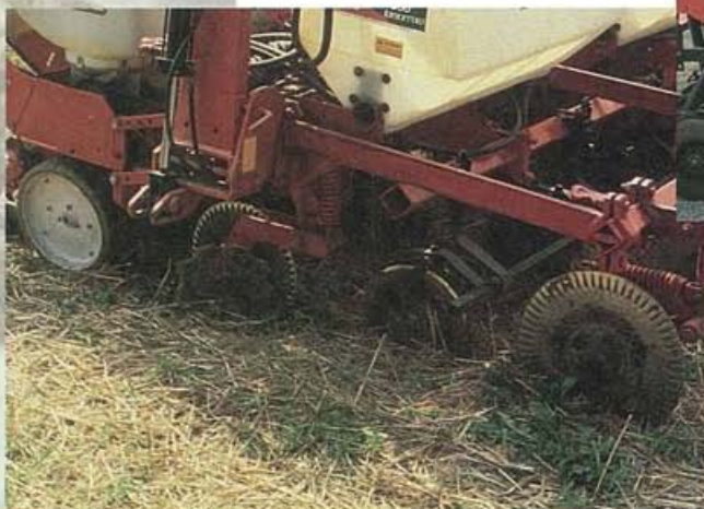
Coulters and trash whippers added to a planter for no-till.
