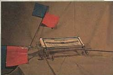
The Contour Gauge is attached to the side window of a truck or tractor. It makes contour layout easier. Drive across the field keeping the bubble centred. Your local extension person may know where one is available.
