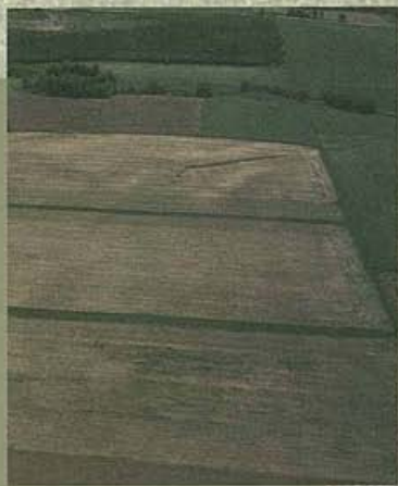
An aerial view of two parallel, narrow base terraces with tile outlet. Designed to break up the slope length, terraces reduce erosion by up to 75% and allow more intense crop rotation.
