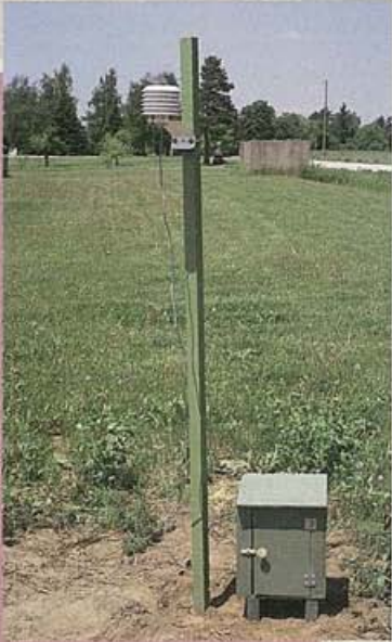
Weather conditions can be monitored by systems such as this TOM-CAST station. The information can then be used to predict some diseases.
