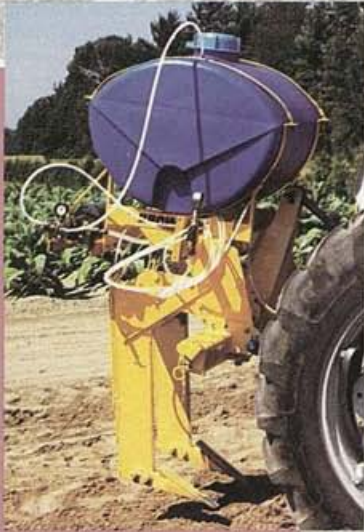
A new fumigation method uses a twin-shank subsoiler to deliver the chemical in a narrow band at three depths.
