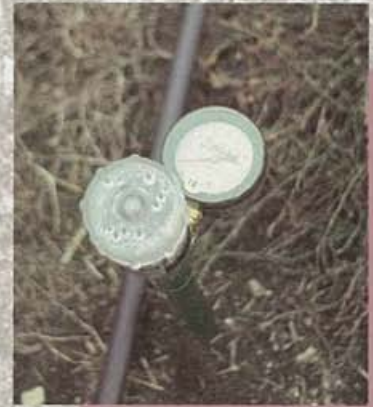
A tensiometer is a valuable tool for scheduling irrigation. An alternative is to use the climate scheduling program which takes into account the moisture holding capacity of the soil and the evapotranspiration losses of the crop.
