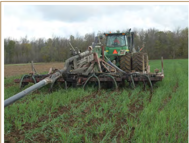
In order to prevent a spill, a direct-flow system must have the capacity to be shut down at a moment's notice.
