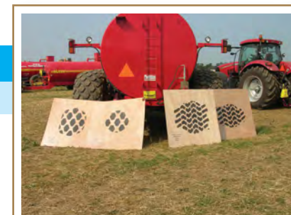
Low-pressure tires on application equipment can increase the surface area of the tire in contact with the soil surface, and help lower the risk of soil compaction.
