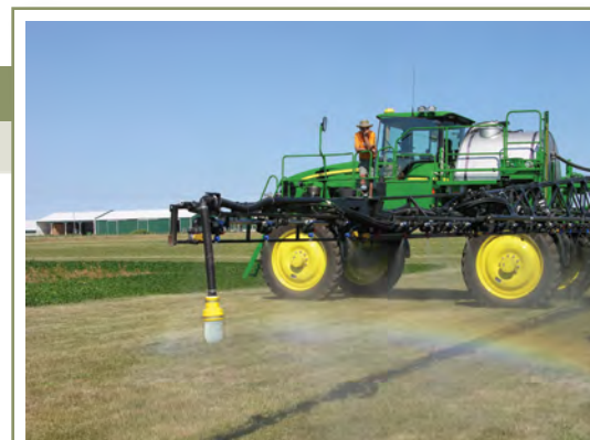
A foam marker at the end of the spray boom will show the edge of the spray line to help ensure continuous spray coverage without excess overlaps.
