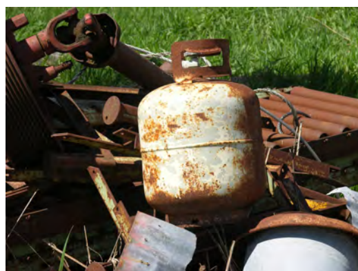
Do not include pressurized containers (e.g. propane tanks) in scrap loads.
