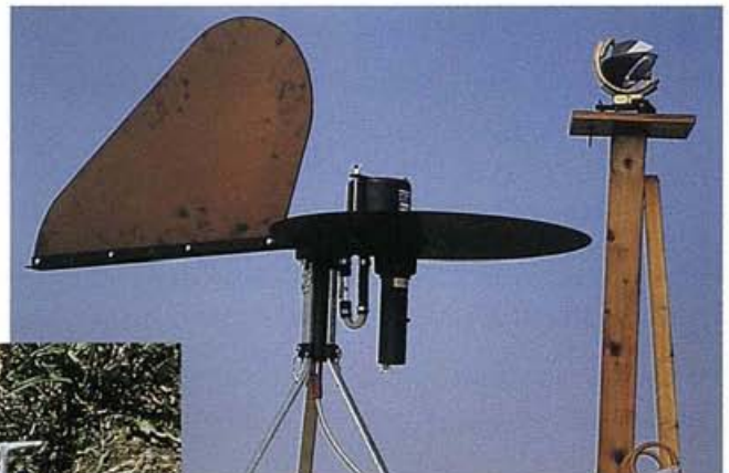
The Hirst spore trap is used to trap spores that initiate plant diseases.
