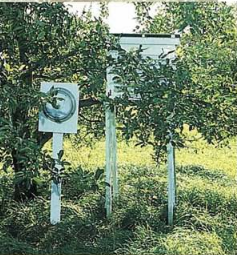
The temperature recorder is kept in a ventilated white box called a Stevenson screen. A second machine, the Dewitt leaf wetness recorder, collects data to predict apple scab infection periods.
