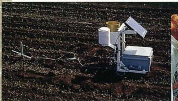
Field weather-station equipment monitors temperature and leaf wetness, and helps to forecast disease episodes on onions.
