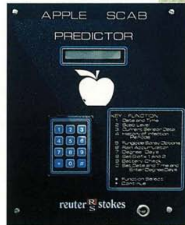
Commercial disease predictors are available. This one measures leaf wetness and temperature, and indicates the occurrence of an apple scab infection period.
