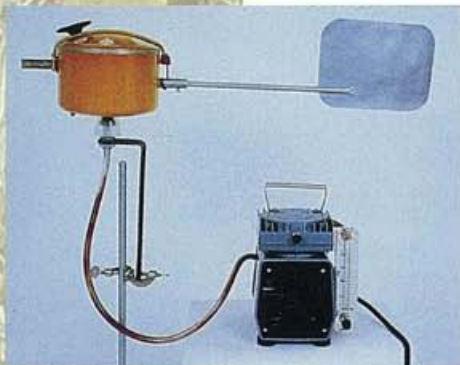
Spores that infect plants and cause disease can be monitored with spore traps.
