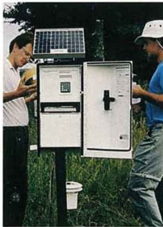
Weather data form a key part of the IPM equation. This machine is used to forecast early and late blight diseases of potato.
