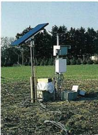
This solar-powered weather station will monitor weather in a vegetable field.
