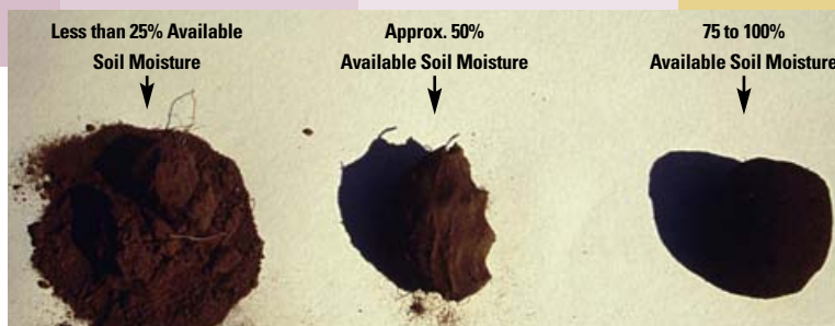
Dry soils are loose or baked. At 100% moisture, a wet outline of water is left on the hand after squeezing.
