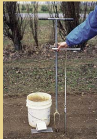
The physical properties of your soils must be known to help make irrigation scheduling work effectively. The technician in this case is taking soil samples to measure water-holding capacity.
