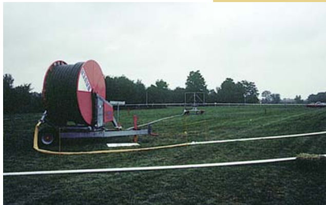
The low-pressure boom traveller system is similar to a travelling gun, except that the gun is replaced by a boom with low-pressure nozzles.
