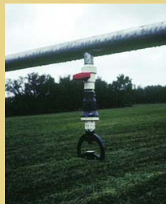
Low-pressure spray nozzles apply fine droplets, making this system useful for delicate crops.
