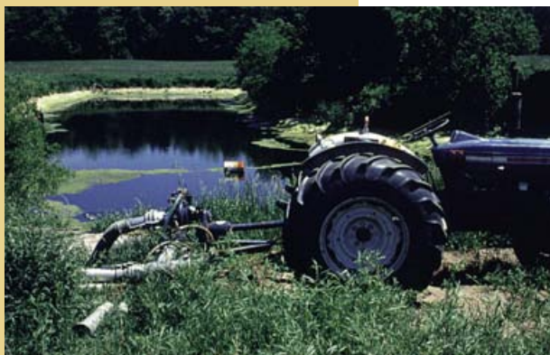
Tractor PTO pumps make good use of existing power sources.
