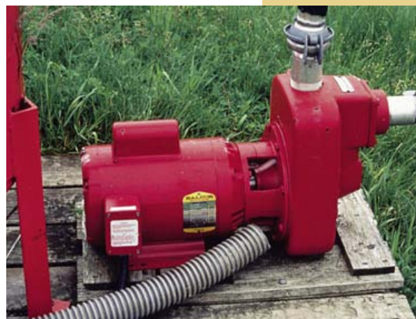
This 3 hp electrical pump is used to supply water to a trickle irrigation system.
