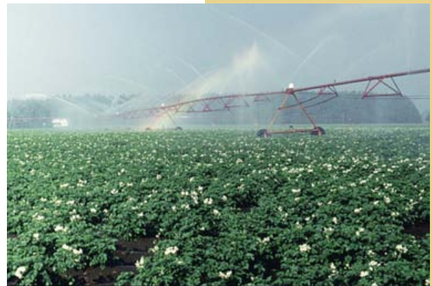
This is an older centre pivot, which consumes more energy because of its high-pressure sprinklers.
