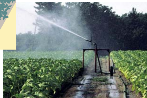
Stationary guns mounted on wheeled frames are also used in the fixed-volume gun hand-move system. Such systems require supervision to avoid runoff on sloping land.
