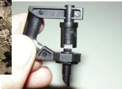
This spray emitter has no moving parts and can be inserted into the line.
