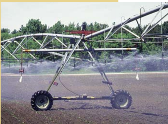
Lateral move systems have a high initial capital cost, but don't require much labour.
