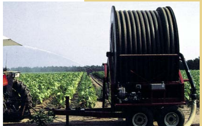
A reel device pulls a mounted gun down the field – irrigating as it goes.
