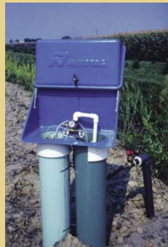
This commercially available sub-irrigation unit will help control the amount of irrigation water supplied to the drainage system.
