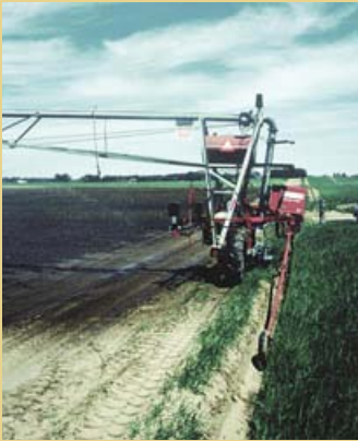
The lateral move system is mechanically similar to the centre pivot, except that it moves sideways across a field in line, irrigating a rectangular section.
