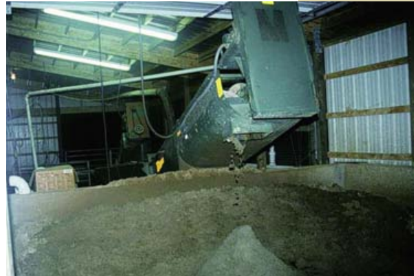
Augers have been developed for sand-laden manure.
