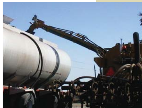
Vacuum loading arms work well for unloading nurse tanks. Where appropriate, include them in your contingency plan, as they're also useful in case of a spill.
