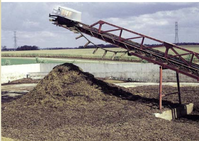
Manure stacker and stable cleaners work well for tie-stall operations, when used in combination with a runoff tank.
