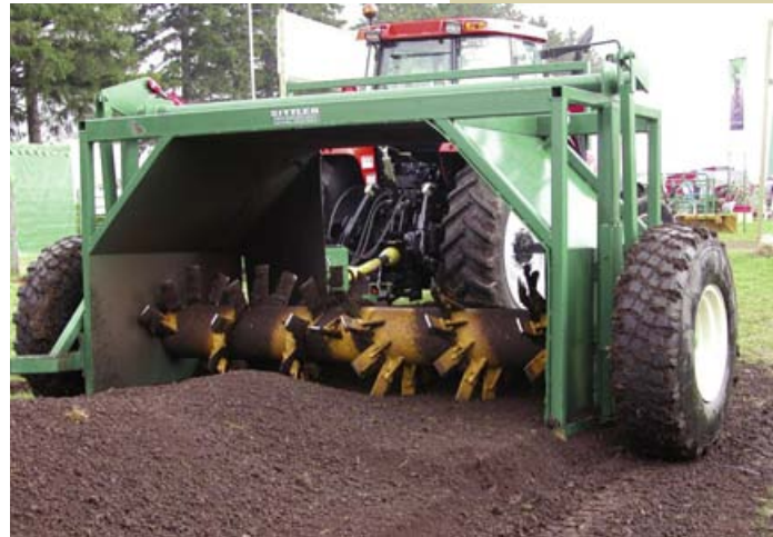
Windrow composters can be used to accelerate the composting process.
