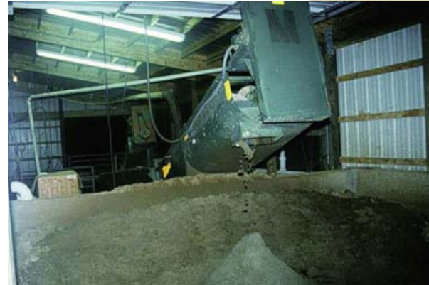
Augers have been developed for sand-laden manure.
