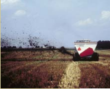
Side-slinger box spreaders work best for poultry manure or other materials with a very low moisture content.
