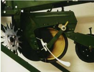
Seed firming devices can improve seed-to-soil contact.
