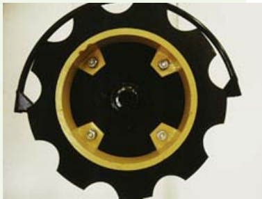
Notched disc blades work well as markers in hard soil and heavy residue conditions. The one shown includes a depth band.
