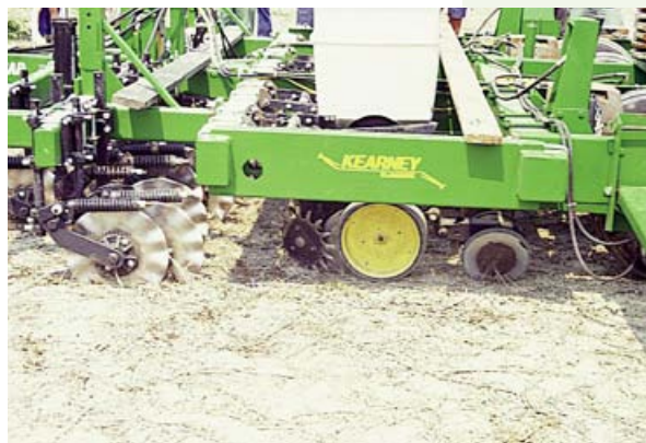
Many ridge tillers are no-tilling on the ridge with the 2-coulter and row cleaner setup.
