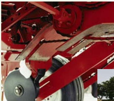
Trash guards protect planting equipment from damage by lodged corn stalks.
