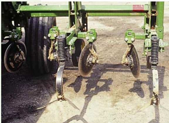
High clearance residue cultivators may be used for no-till weed control and in the ridge till system.
