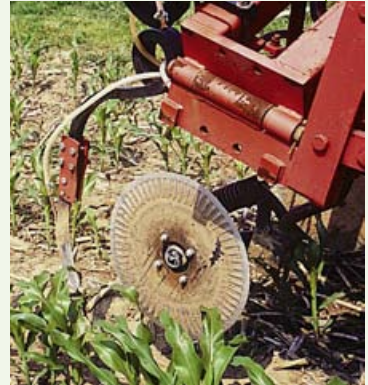
A coulters in front of the knife cuts residue and improves nitrogen placement.
