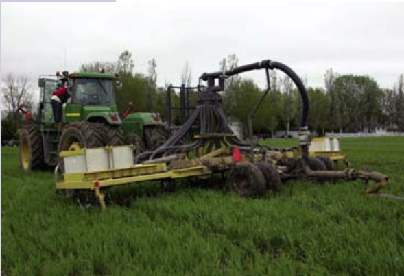
Injection methods place the nutrients in the root zone to improve availability for crop use.
