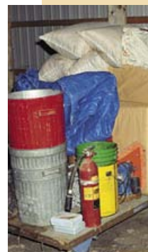
This homemade spills kit uses readily available materials for diking, containing, absorbing and disposing of contaminated materials from a spill.
