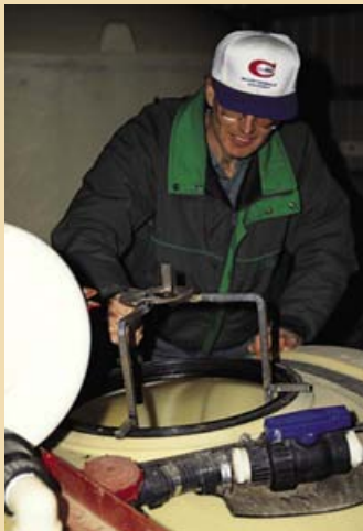
An anti-backflow device may be as simple and effective as this farmer's innovation. The sprayer modification is placed over the tank opening and the hose is attached to the device during filling.
