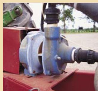
Flush the pump daily.
