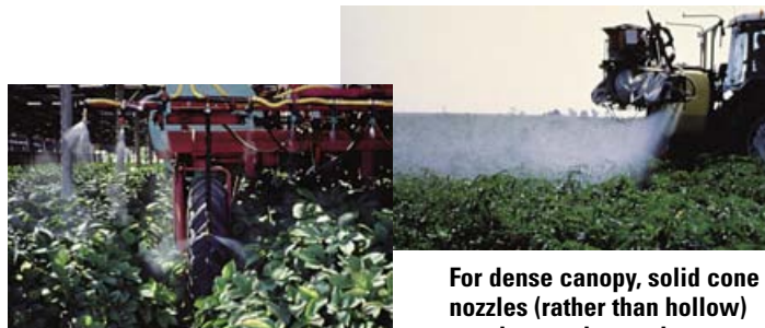
NOZZLE CONFIGURATION. Hitting the target may mean changing the configuration of nozzles (e.g., drop nozzle in ginseng for foliar disease control).
