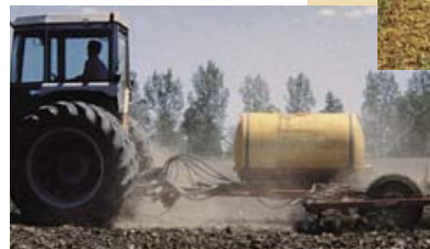
ROW CROPS. For pre-plant operation, the target is the soil surface. Use the nozzle that produces low pressure and large droplets. (Floods or flat fans would work.)
