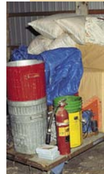
This homemade spills kit uses readily available materials for diking, containing, absorbing and disposing of contaminated materials from a spill.
