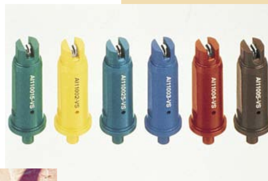
Air induction tips add air to reduce pressure and increase droplet size. They help reduce drift and increase coverage.
