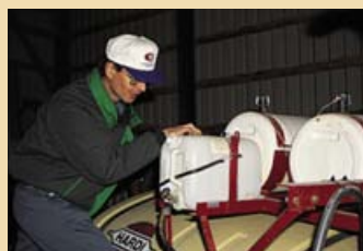
By attaching tanks of water to his field sprayer, this producer is able to rinse out his tank and apply rinsate to the sprayed fields.
