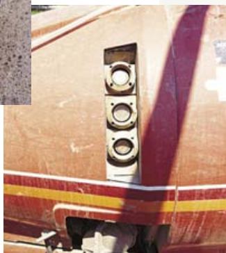
This tree-sensing sprayer uses reflected light to sense orchard tree presence as it proceeds through the orchard.
