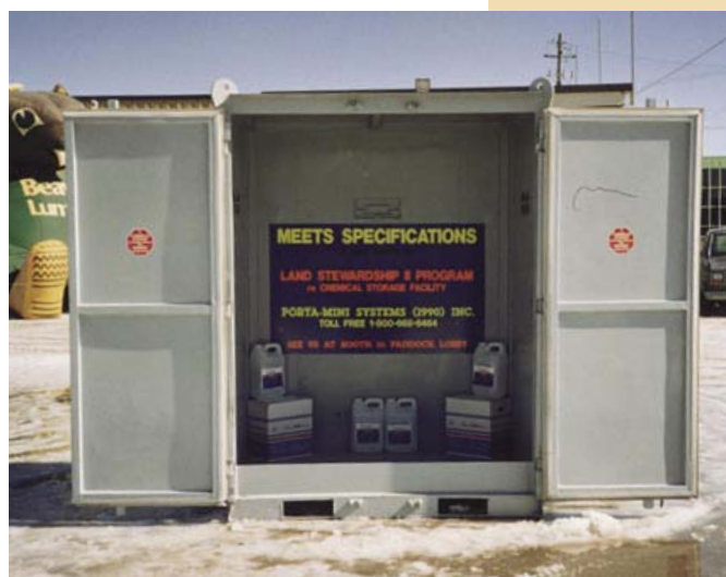
Vertical cabinets can make suitable storages, provided they are vented, locked, and will contain leaks.
