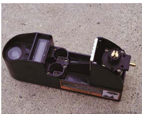
Vegetation-detecting sprayers are also available. Infra-red detectors can sense the presence of weeds. Nozzles turn on and off to spray sensed weeds.
