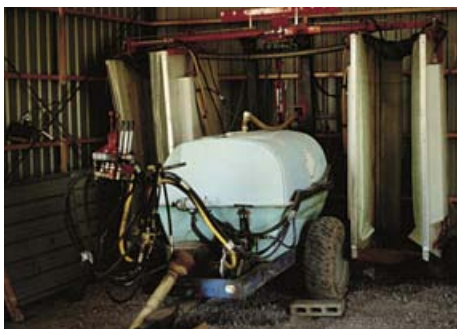
Recycling sprayers reduce drift and increase sprayer effectiveness by using walls and troughs to recycle spray mixture.
