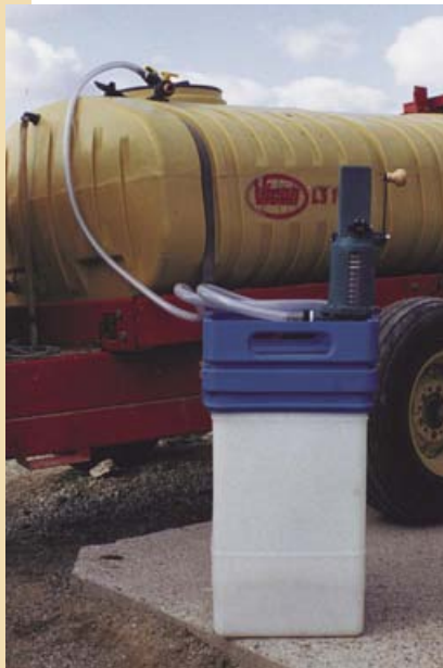
This volumetric hand pump will help producers add precise volumes and avoid splashes and spills.
