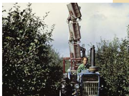
Air curtain sprayers have compartments of nozzles and hydraulic arms to reduce nozzle-to-target distances and attain better canopy penetration.
