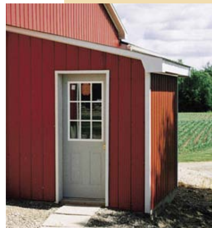
Built-on storages require ventilation to the outside, an outdoor entrance, and proper firewalls.
