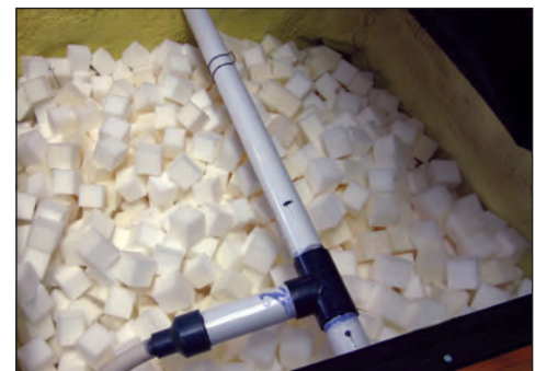
Synthetic media — foam cubes (top view).
