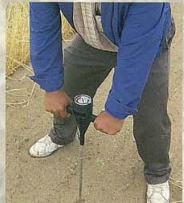
Penetrometers are used to estimate soil strength and to look at the different responses in experimental treatments. Penetrometers give a good estimate if used properly, although a flexible tile probe works just as well, particularly in farm fields. See "Detecting Compaction", page 36.
