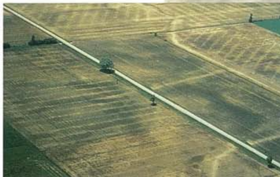
Subsurface drains remove excess water from the soil profile.
