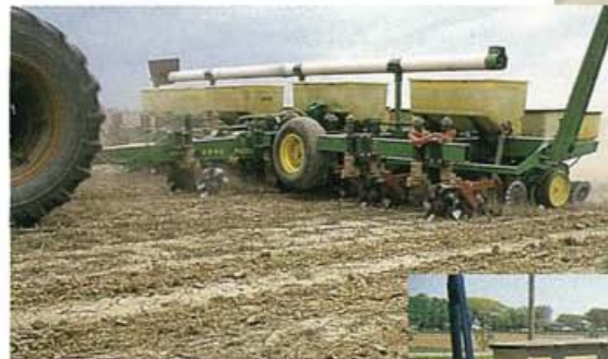
No-till planters take a variety of forms, from three or more coulters with trash whippers to none. Most systems do move residue and perform some tillage.
