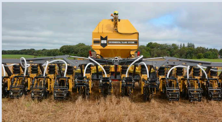
Figure 9. Some strip-tillage machines, such as this coulters-based unit, come equipped with dry fertilizer delivery systems.
