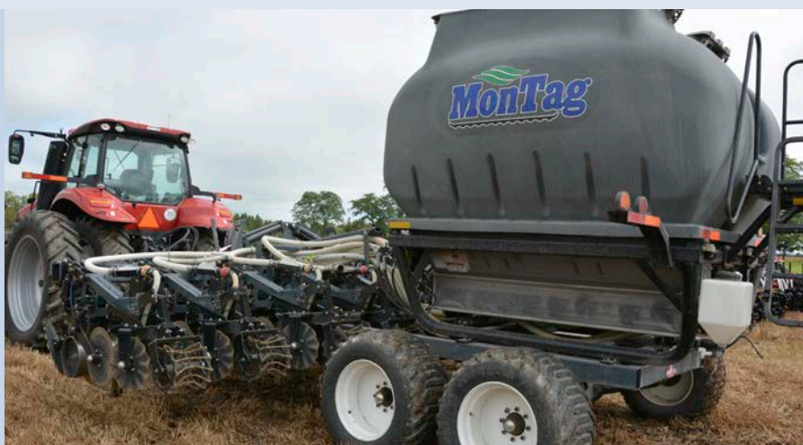
Figure 10. Air carts can also be after-market additions to strip-tillage equipment, as seen in this example.
