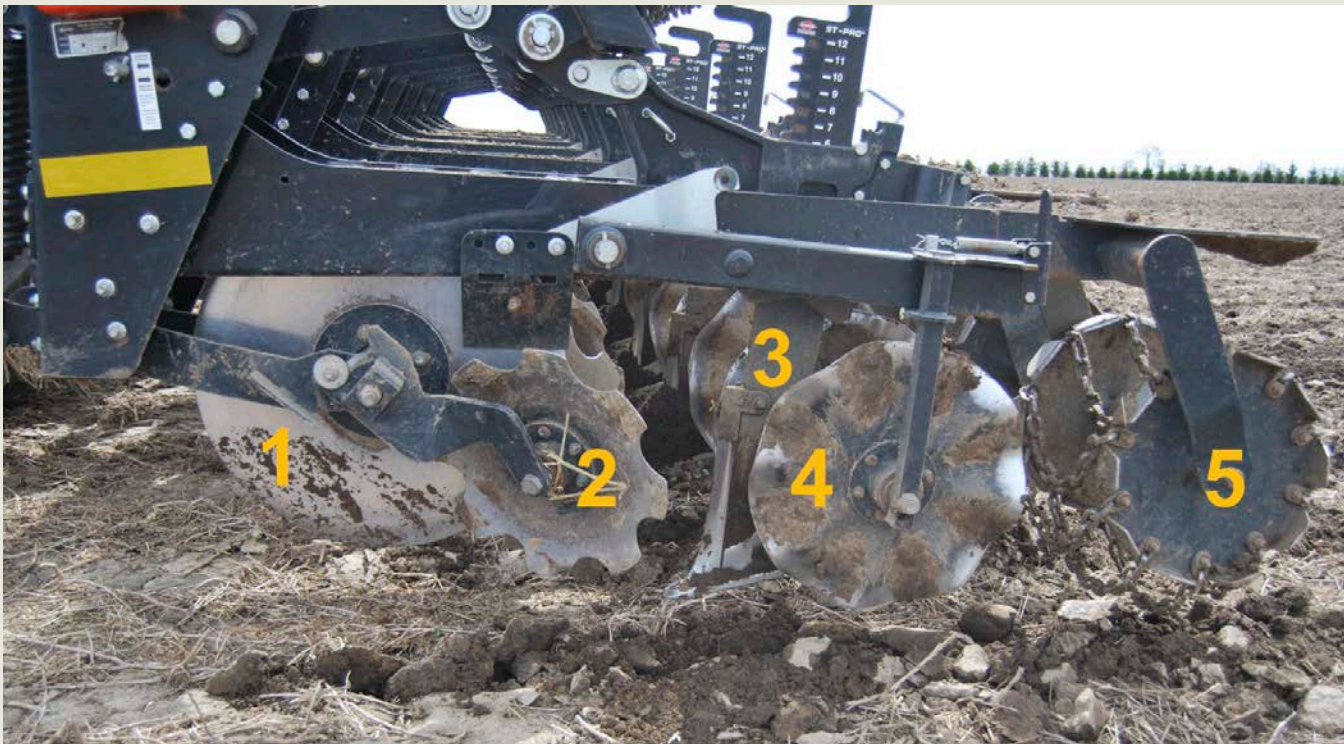
Figure 3. An example strip-till unit. From left to right, each unit on this strip-tiller includes: 1) a cutting coulters, 2) residue cleaners, 3) a shank, 4) working/containment coulters and 5) a rolling basket.
