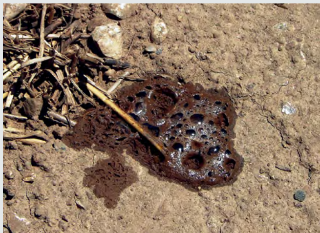
When 10% hydrochloric acid (HCl) is applied to soil and bubbles and foam appear, this indicates that calcareous (high lime) parent materials or a mixture of topsoil, subsoil and parent materials are present at the soil surface.
