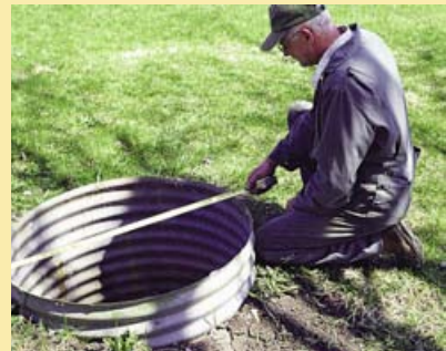
The inside diameter of the casing can easily be measured by the landowner.
