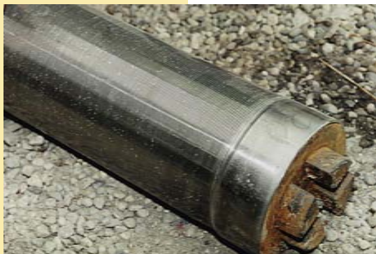
Shown here is a stainless-steel well screen. The screen holds back sediments in the aquifer, while allowing the water to flow into the well casing.
