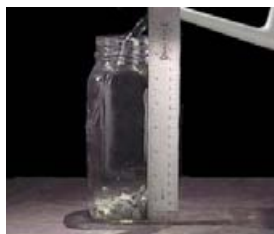
Water added to bentonite.
